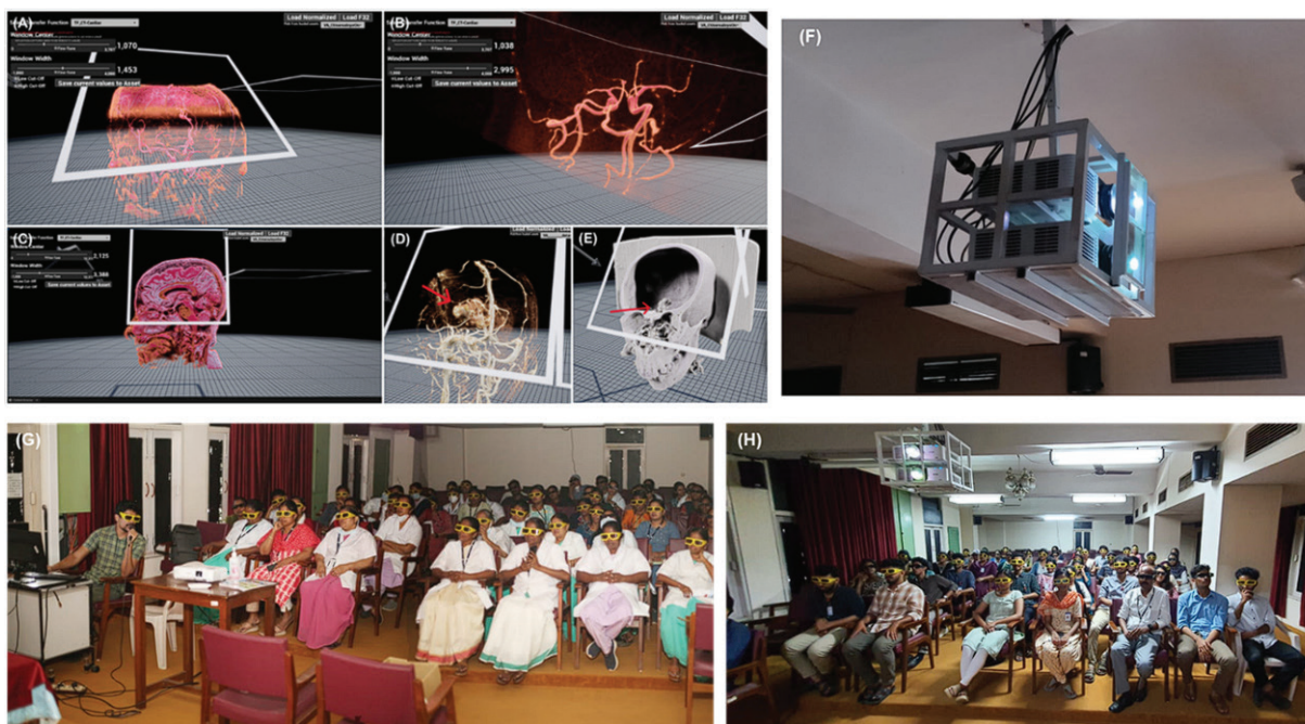
Figure 1. Surgical planning system at SCTIMST: (A-E) Images of the renderings of different anatomical regions using the developed tool, (F) Photograph of 3D dual projector setup, and (G-H) clinicians and students viewing images using 3D glasses.
