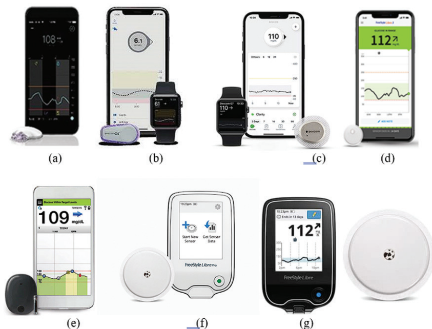
Figure 1. Types of CGM systems ((a) Guardian Connect (b) Dexcom G6 (c) Dexcom G7 (d) FreeStyle Libre 3 (e) Eversense (rt-CGMs) (f) FreeStyle Libre Pro (P-CGM) (g) FreeStyle Libre (isCGM))
